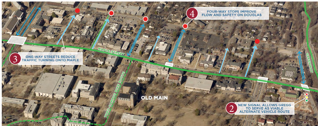
Figure 6. An overview of proposed improvements to traffic flow and safety.
