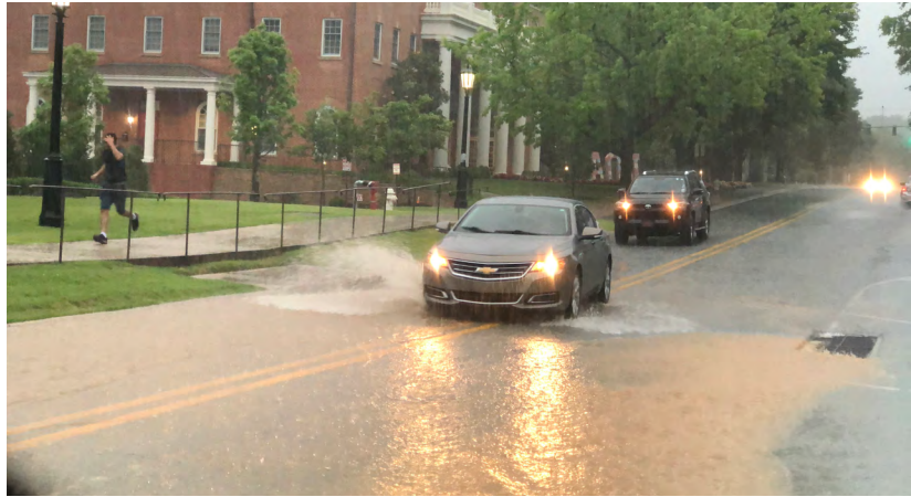
Figure 21. Inadequate stormwater infrastructure on Maple St. is overwhelmed by a common ½ inch rain event.
