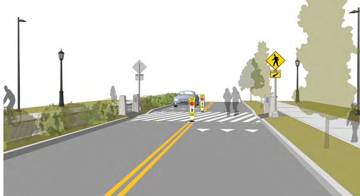
Figure 18. Upgraded crosswalk designed with pedestrian safety features. (UA Community Design Center, 2019)
