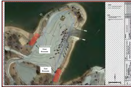
Fig 2. Illustrates the placement of the bioswales that will filter runoff water as it exits the parking lot. (Hodges, 2015)
