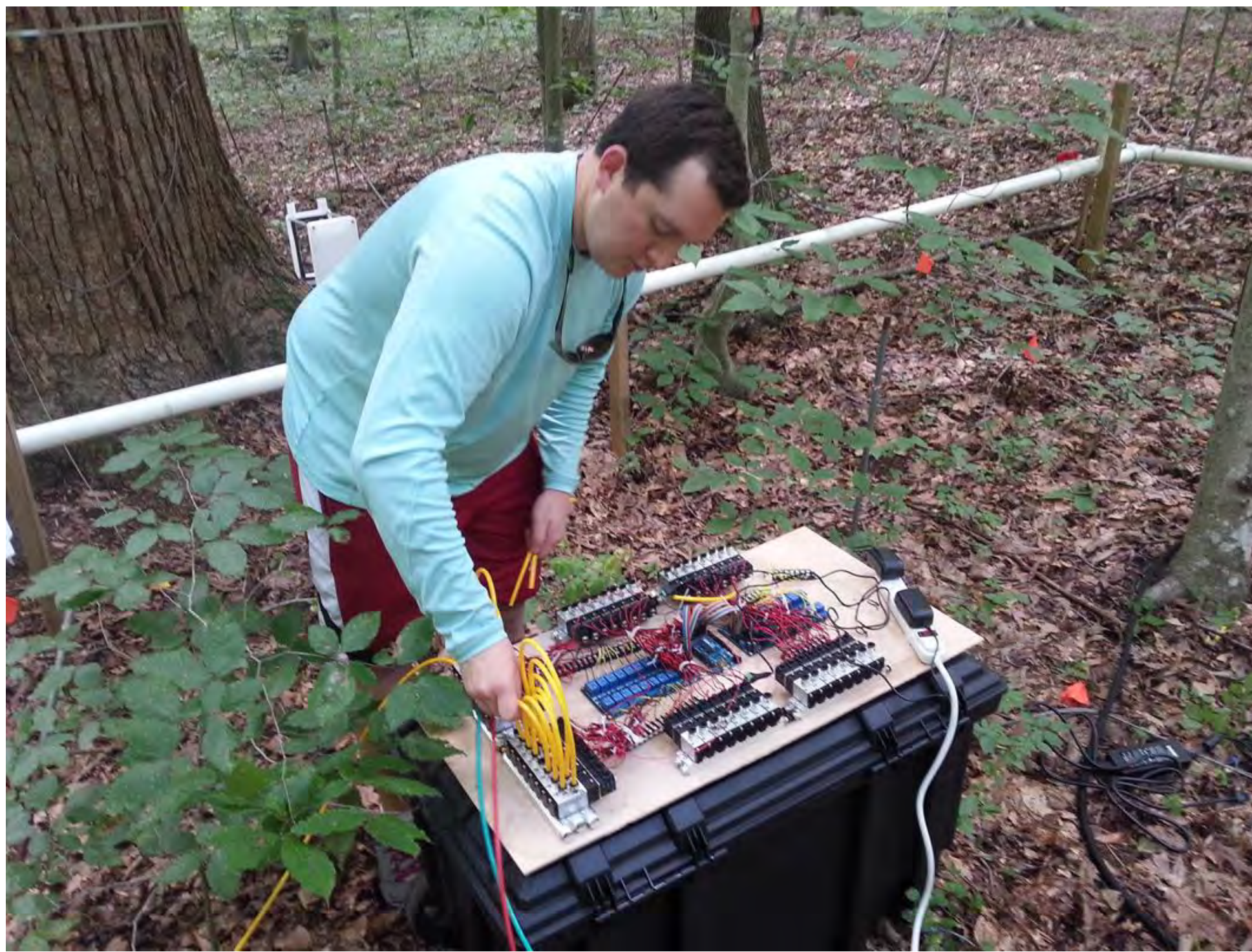
Fig 1. Setting up the tubing to our main board that cycles the air sample from the tree chamber through the gas analyzer and back. All chambers were programmed to open and close using open source hardware called Arduino Mega.
