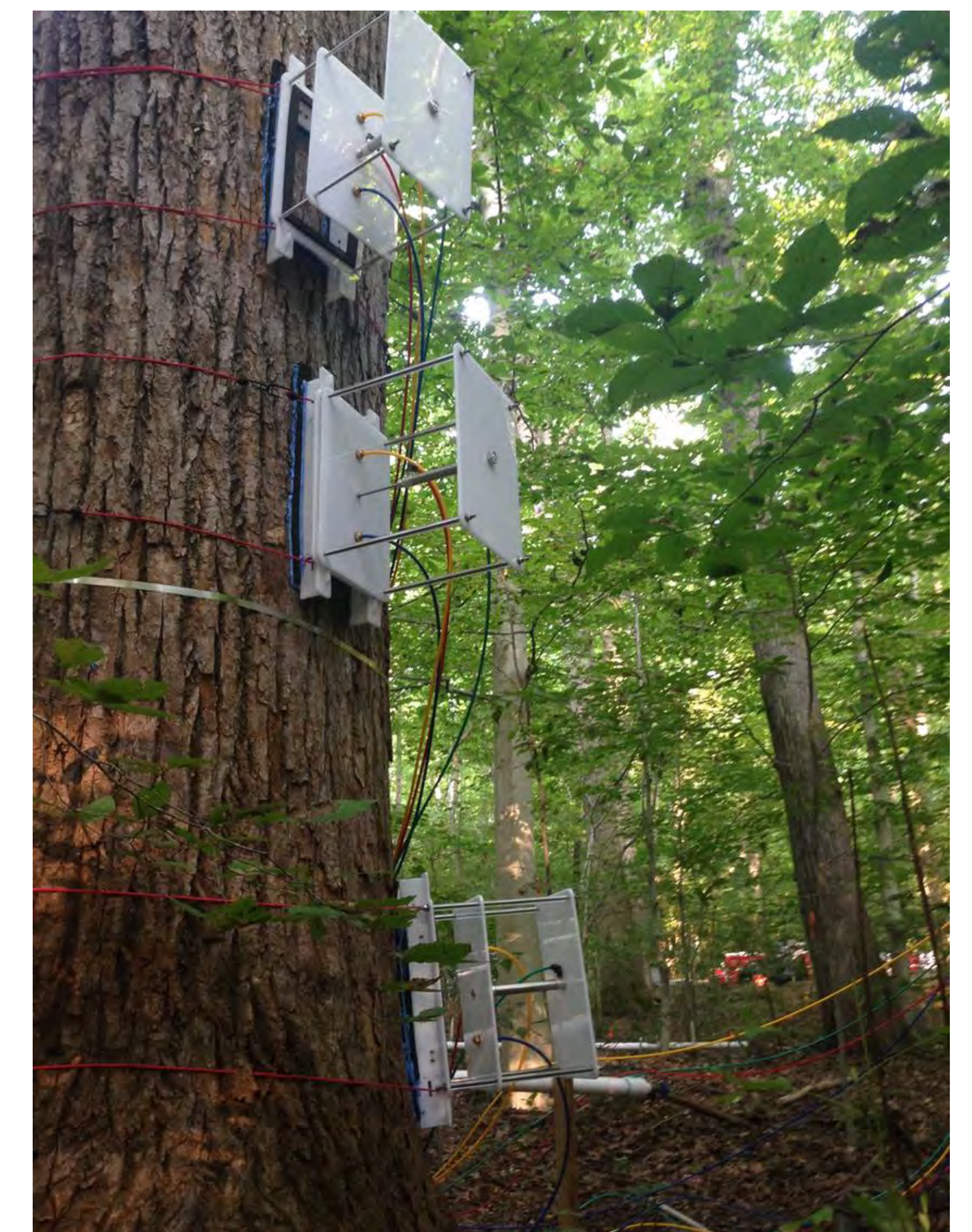
Fig 6. View of the automatic chambers during a sampling run on a Tulip Poplar tree at heights of 75 cm, 165 cm and 245 cm. The middle chamber at 165 cm is closed and cycling air through the gas sampler.
