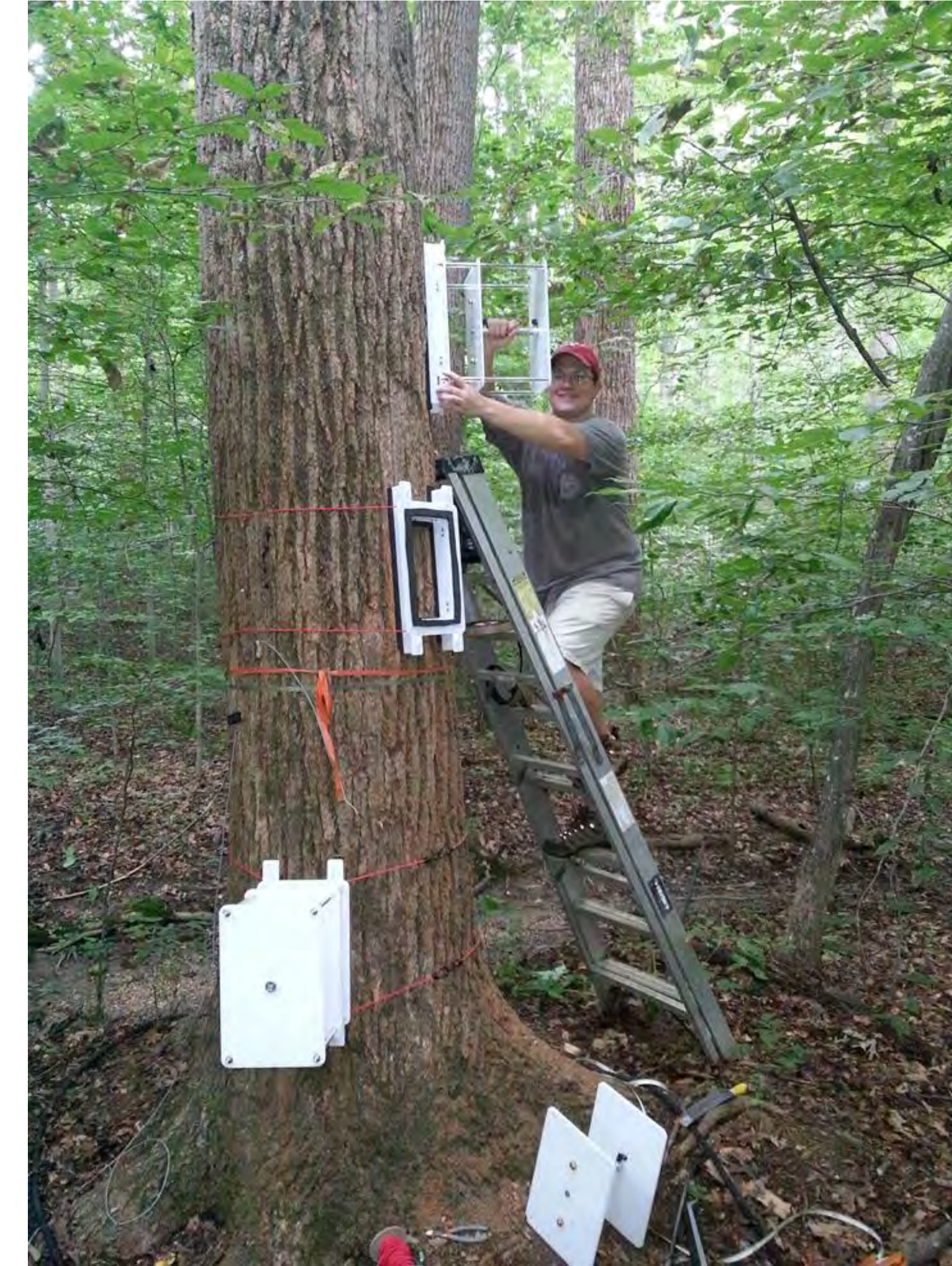
Fig 3. Installing the monitoring chambers on one of the Tulip Poplar trees. Chambers were custom designed, cut and sealed on the trees.
