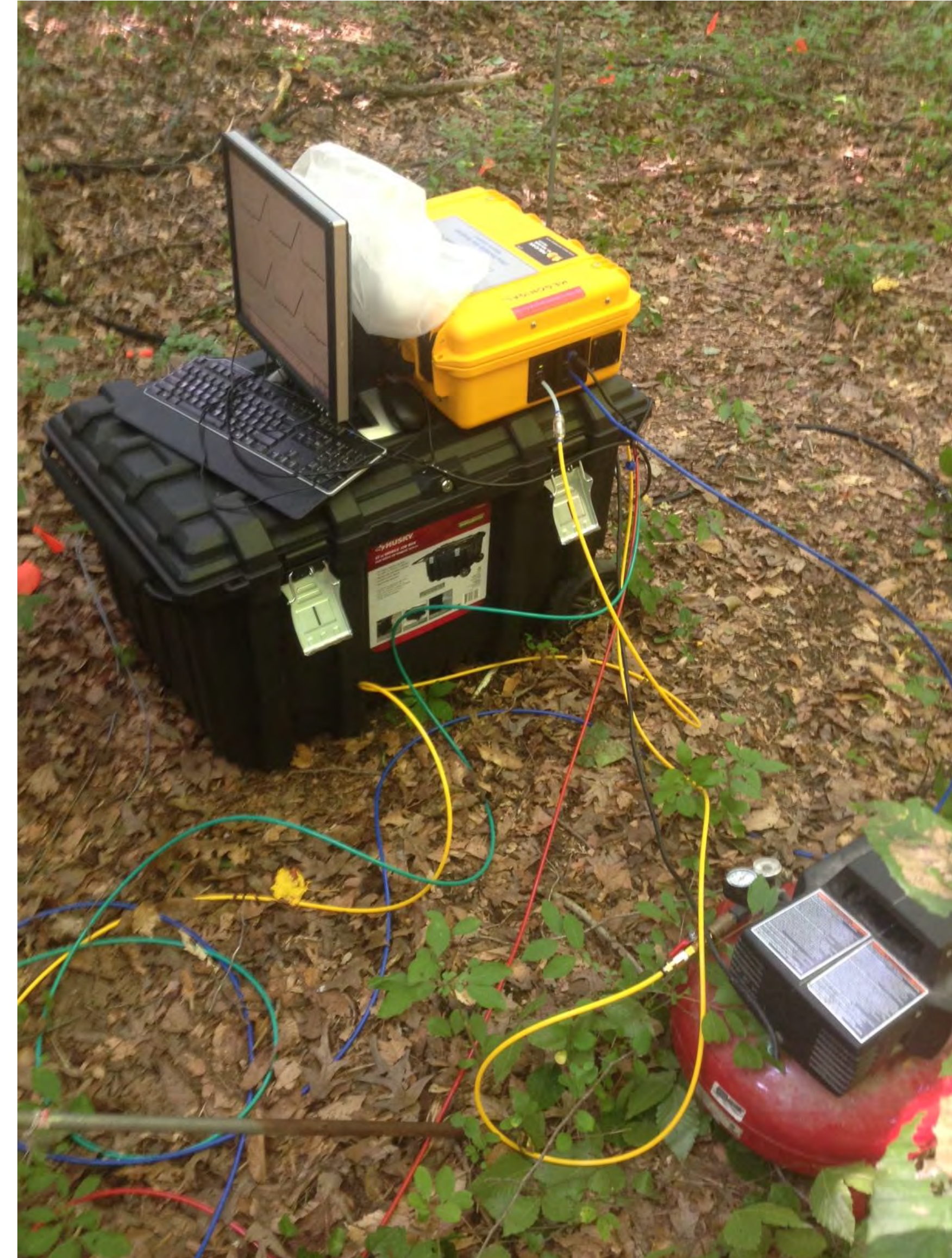
Fig 2. A view of the portable gas analyzer (yellow). It uses Off-Axis Integrated Cavity Output Spectroscopy (OA-ICOS) to monitor in real time the concentrations of methane, carbon dioxide, and water vapor of the gas pumped through its sampling chamber.
