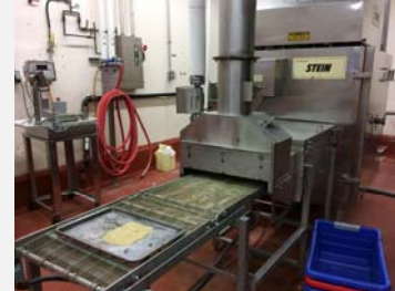
Figure 3. Impingement Oven - Poultry Pilot Processing Plant
