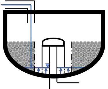
Water reaches bottom level and begins to fill up with water, repeating the process
