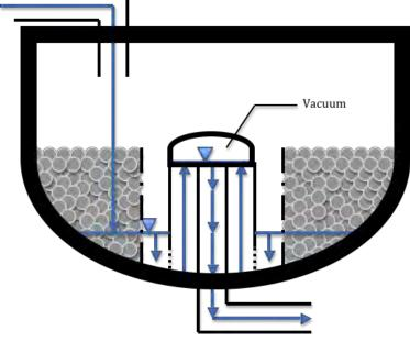
Siphon created and water is forced from the grow bed to drain out to fish tank
