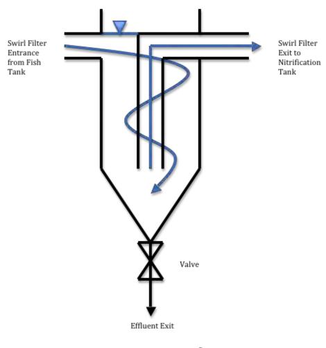
The water is then sent to an nitrification tank by gravity. This environment consists of bacteria called nitrosomas, which convert the ammonia rich water into nitrite, and nitrobacters, which convert the nitrite into nitrate. Nitrate is a natural fertilizer for plants.
